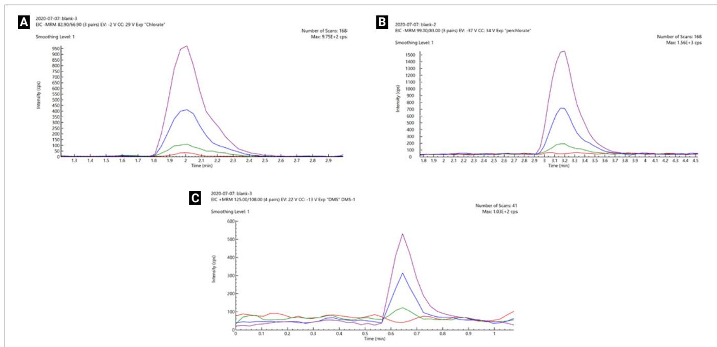
Figure 8: Overlay of the 3 metabolites quantifier fragments at different calibration levels, red= 0 µg/L, green= 0.01 µg/L, blue 0.05 µg/L and purple= 0.1 µg/L for A. chlorate, B. perchlorate and C. DMS.
