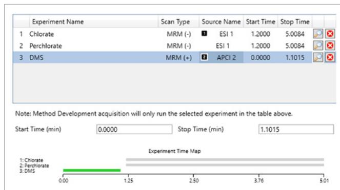
Figure 2: View from the Simplicity 3Q Software Platform of how the MS method is setup. DMS is first measured with APCI from 0 - 1.1 minutes. Then chlorate and perchlorate are measured from 1.2-5 minutes.
