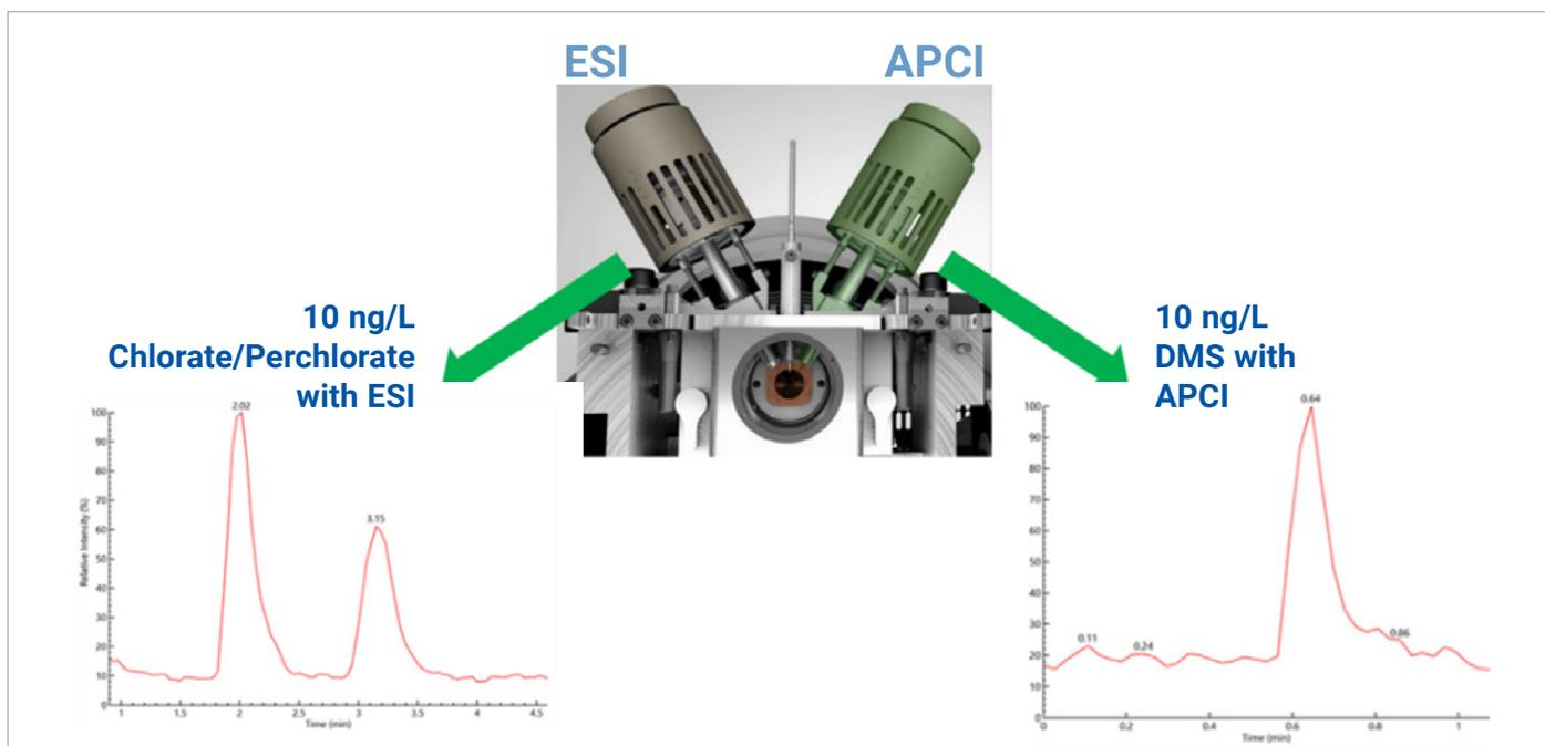
Figure 6: Shows that switching between ESI negative mode and APCI positive mode is possible in a single run without losing key sensitivity of the metabolites. On the left is a chromatogram of chlorate and perchlorate in ESI negative mode and on the right is DMS in APCI positive mode.
