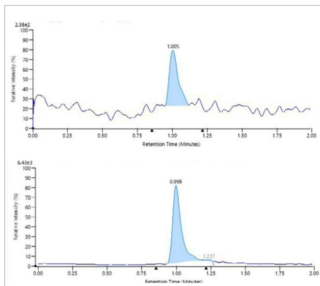
Figure 5: Chromatogram of a drinking water sample with a positive find of acrylamide at 0.02 µg/L, left pane is the quantifier fragment and right pane is the isotopically labelled internal standard. The % RSD (n=5) was 5.8 %.
