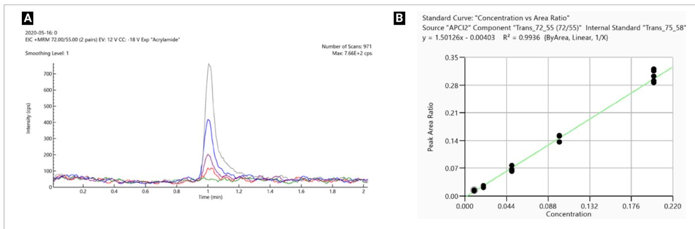
Figure 4: Overlay of acrylamide quantifier fragment at different matrix-matched calibration levels, green= 0  $\mu\text{g/L}$ , red= 0.01  $\mu\text{g/L}$ , purple= 0.02  $\mu\text{g/L}$ , blue 0.05  $\mu\text{g/L}$  and grey= 0.1  $\mu\text{g/L}$ . B. Calibration curve for acrylamide (0.01-0.2  $\mu\text{g/L}$ ) with an  $R^2$  value of 0.9936 with five replicates per calibration standard.
