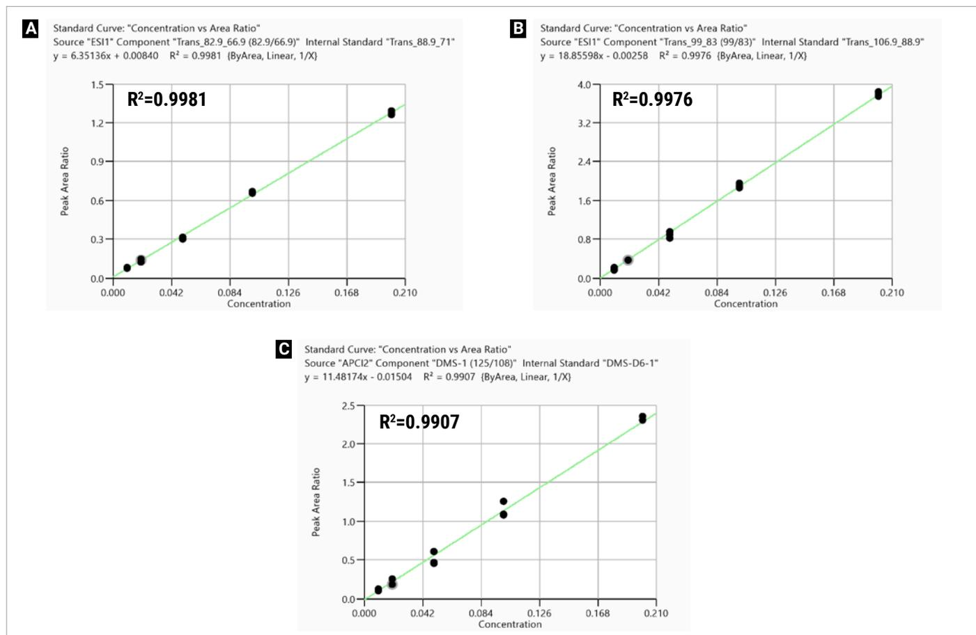
Figure 7: Calibration curves for the 3 metabolites in concentration ranges of 0.01-0.2 µg/L with an  $R^2$  values all > 0.99 for A. chlorate, B. perchlorate and C. DMS.
