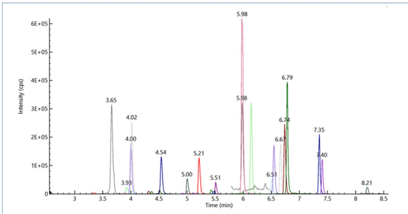
Figure 2: Extracted ion chromatograms of the less polar analytes in a spiked milk sample.
