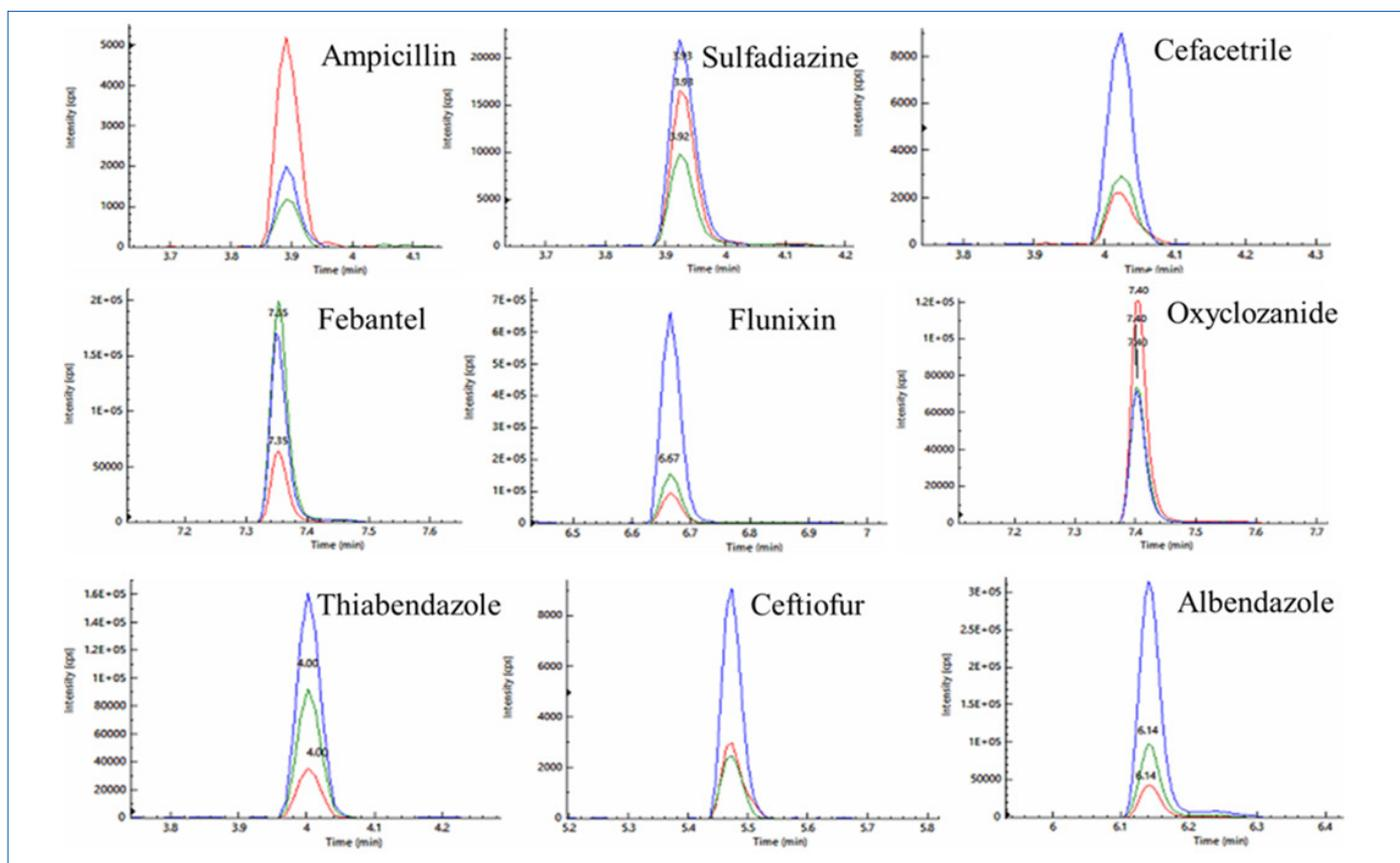
Figure 5: Overlapped three MS/MS chromatograms of some less polar analytes spiked at 5 µg/kg in milk.
