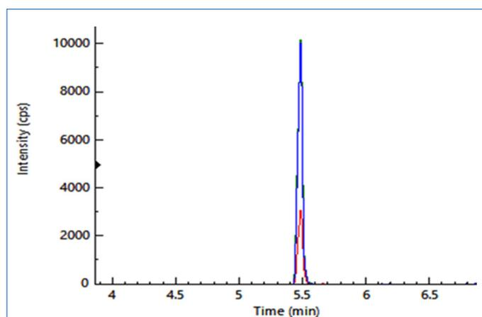
Figure 4: MS/MS chromatograms of diminazene in a spiked milk sample separated using the mixed mode Obelisc R column.
