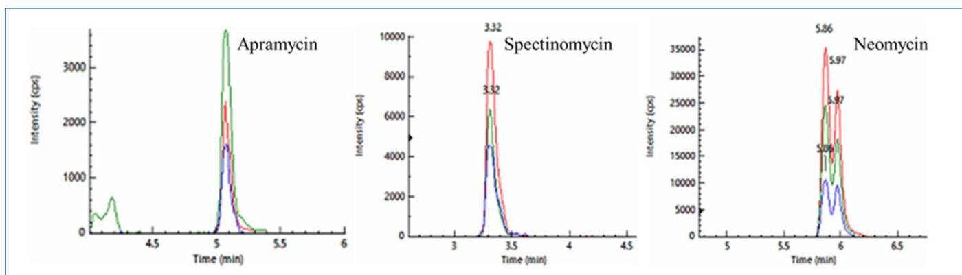
Figure 6: Overlapped three MS/MS chromatograms of aminoglycoside antibiotics spiked at 50 µg/kg of apramycin, 100 µg/kg of spectinomycin, and 1000 µg/kg of neomycin in milk.
