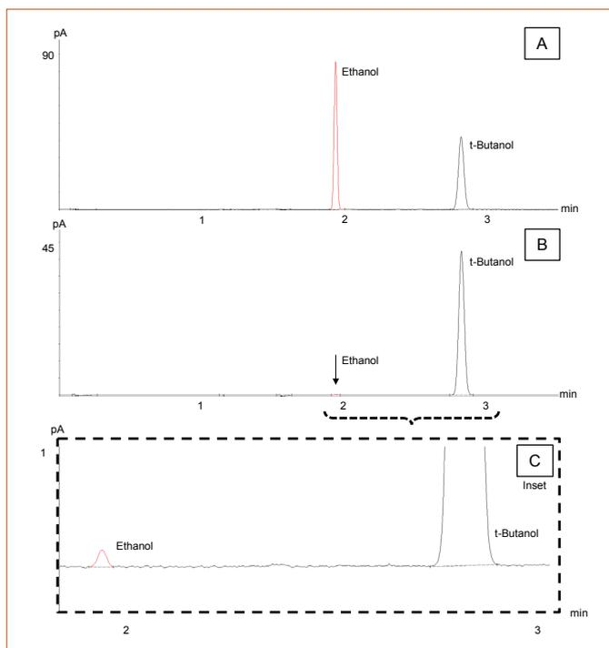
Figure 2. Calibration standard chromatograms of (A) ~1.0% vol/vol standard, (B) ~0.0020% vol/vol standard, and (C) inset of low-level standard highlighting signal/noise at low end of calibration curve.
