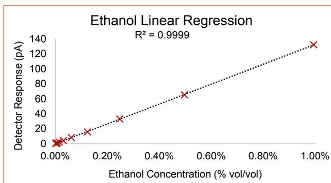
Figure 1. Calibration curve for ethanol by headspace GC/FID.
