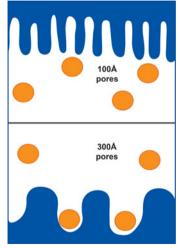
Representation of small pore particles ( $\sim$  100 Å) vs. wide pore particles ( $\sim$ 300 Å). Smaller pores do not allow most proteins to enter the pores, which limits interaction.
