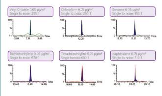
Recommended Column: Elite-624, 60 m x 0.25 mm x 1.4  $\mu\text{m},$  Part No. **N9316006**
