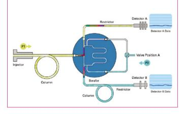
Swafer can be installed in any Clarus 580/500 or 680/600 GC with programmable pneumatic control (PPC).
