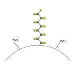
Fluorinated phases are able to perform many unique and difficult separations which cannot be performed on the best available C18 columns. Traditionally, fluorinated phases have suffered from poor column lifetimes, unstable baselines and column bleed, especially when used with mass spectrometry (MS). Epic FO LB has been stabilized to provide low column bleed, increased lifetimes, better pH stability, and superior LC-MS performance.
