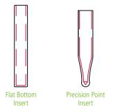
Our vial inserts are made from the same Type 1 borosilicate glass as our vials and can be used for maximum sample extraction when handling micro volumes. Extend the usability of your Standard or PureView 2 mL vials with the addition of a micro volume insert. Simply select the vial insert that matches with the neck ID of your vial.
