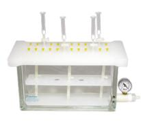
the stationary phase, metered by the stopcocks, to control the speed of the extraction process and the sample flow. Waste and wash solvents are discarded and analytes are collected in sample tubes below the manifold completing the extraction. For your convenience, manifold kits are supplied in either 12 position or 24 position configurations.
