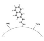
and performs well for diastereomer separations and non-polar compounds. The unique properties of Epic Naphthyl places its selectivity between graphitized carbon and alkyl type stationary phases.
