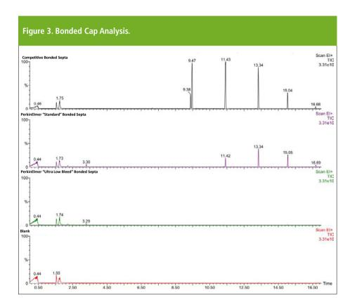
The GC comparison, above, compares a competitive brand of septa to PerkinElmer's standard and ultra-low bleed septa products. The level of siloxanes bleed identified in the competitive product is clearly at a much higher level compared to our septa.
