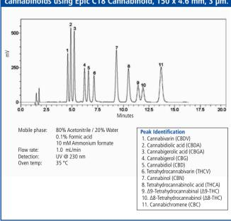
HPLC analysis of 11 major and most frequently observed cannabinoids using Epic C18 Cannabinoid, 150 x 4.6 mm, 3 µm.
