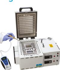
condition each tube individually on your thermal desorption instrument. This takes time – especially if you have several tubes to condition – and also ties up your instrument which could be used for more important analysis. Or, a better more efficient alternative is to condition your tubes in a separate oven.
