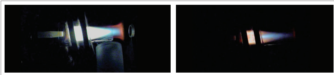
Figure 1. The figure on the left shows the angled base of the plasma which coincides with the angled shape of the load coil. The figure on the right shows the upward tilt of the axial channel and plasma tip as well as the differences in plasma density above and below the central channel.
