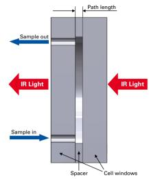
pumping a thin film of the sample between two parallel windows of Calcium Fluoride (CaF<sub>2</sub>). The instrument measures the Infrared absorption of the components of interest in the milk by passing Infrared energy through the windows and sample to a detector.
