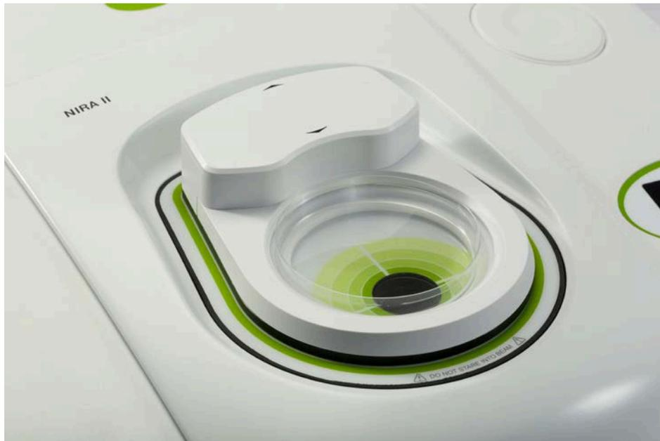
**Figure 14 NIRA II Sample Spinner in position over sample window**
