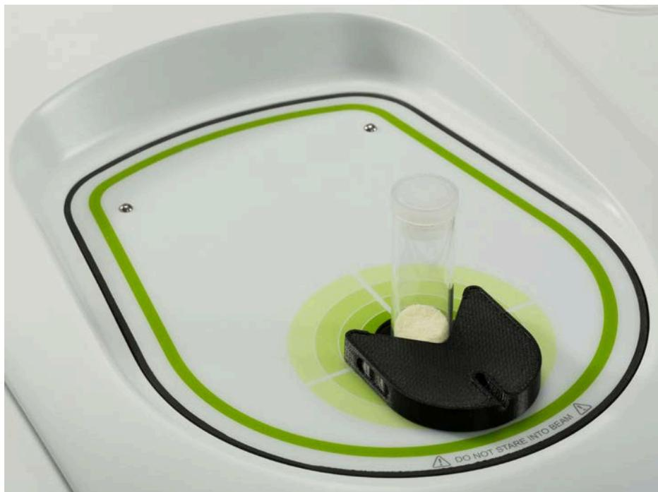
**Figure 6 Sample Alignment Tool in use**
