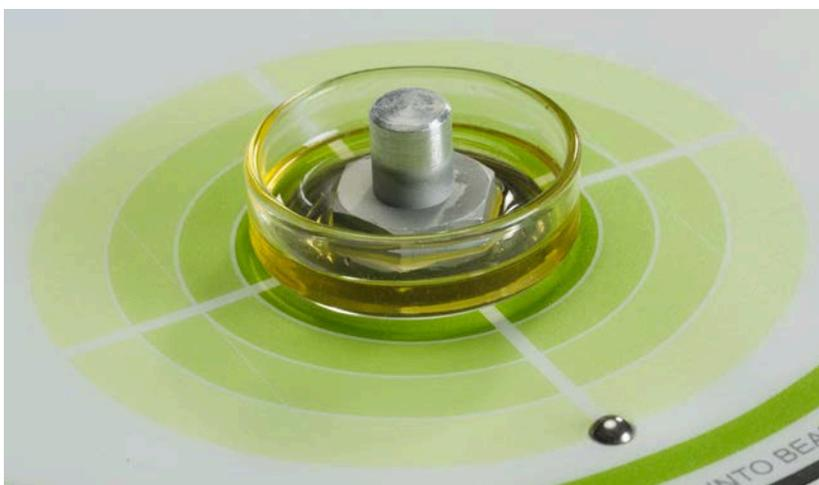
**Figure 24 Liquids transmittance accessory in position**
