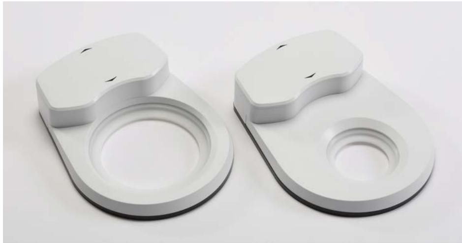
**Figure 12 NIRA II Sample Spinners for 100 mm (left) and 60 mm (right) Petri dishes**
