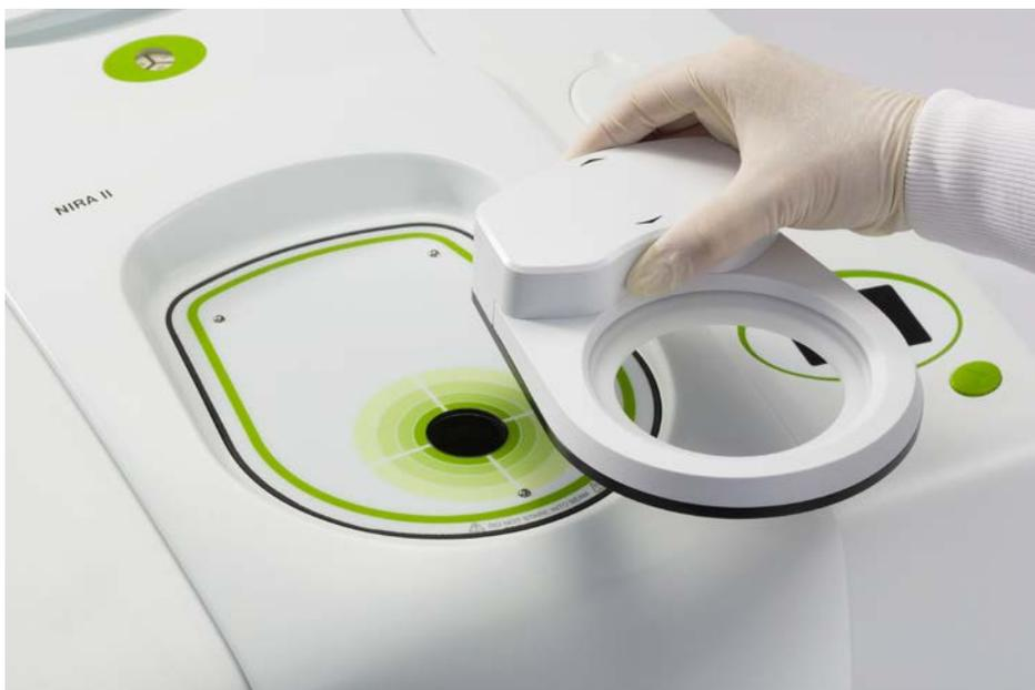
**Figure 17 Removing the Sample Spinner from the NIRA II top plate**
