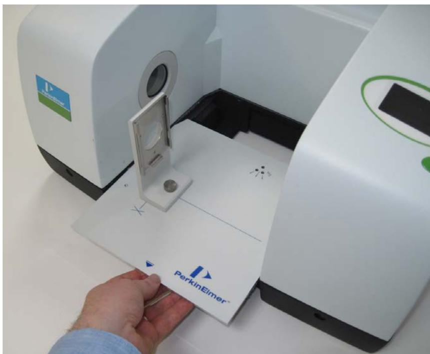
**Figure 8 Removing the basic sample slide**
