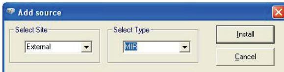
The selection in the Select Type pane defines the default wavenumber range of the instrument, which can be edited in the Spectrum software. The effective scan range of your instrument will depend on its configuration, such as the detector and the beamsplitter.
