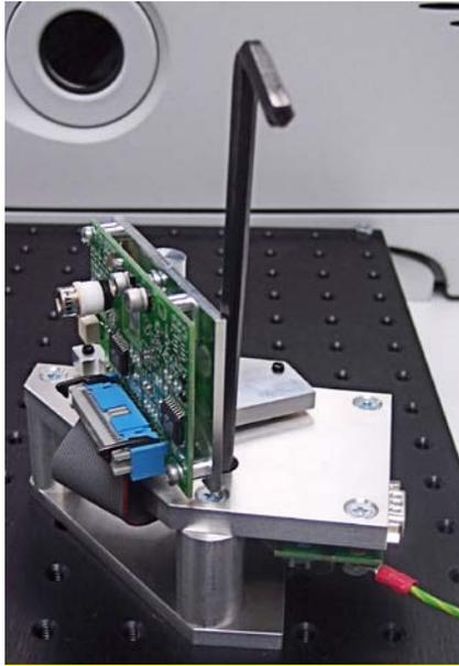
**Figure 8 Fixing the detector/preamplifier module to the bench**
