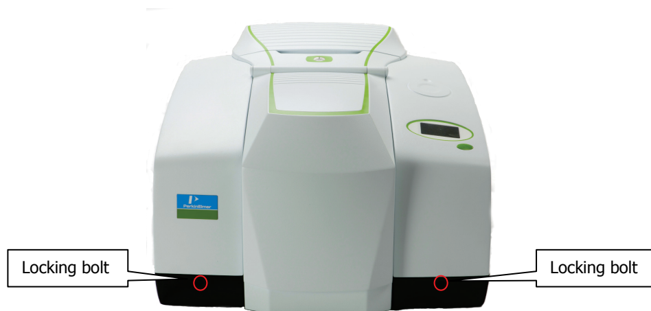
Figure 33 Main cover locking bolts
