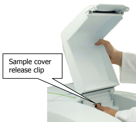
Figure 24 Removing the sample compartment cover
