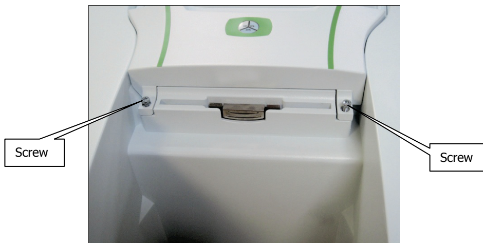
Figure 25 Captive screws securing the desiccant cover
