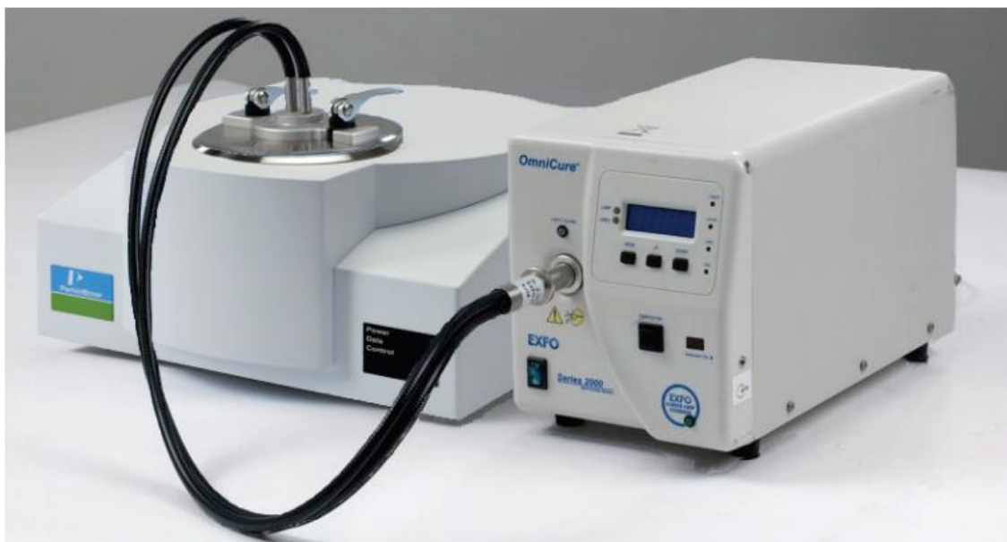
Figure 2 Thermal analyzer connected to a DSC-Photocalorimeter
