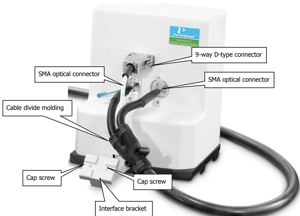
**Figure 6 Connecting the probe cable to the Sample Area Interface**
