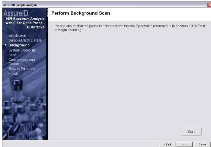
6. Holster the probe and then press the probe trigger, or click **Start**, to begin data collection.
