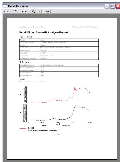
The report shows the results of the analysis. In this example, the spectrum collected for test 003 is not the material specified.
