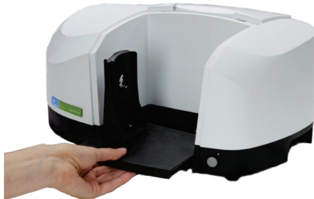
**Figure 2 Removing the standard baseplate**
