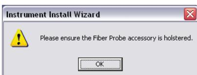
5. Holster the probe, making sure that the Spectralon reference material is in place, and then click **OK**.
