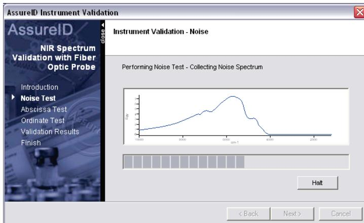
The probe display shows 'Collecting Noise Spectrum'.
