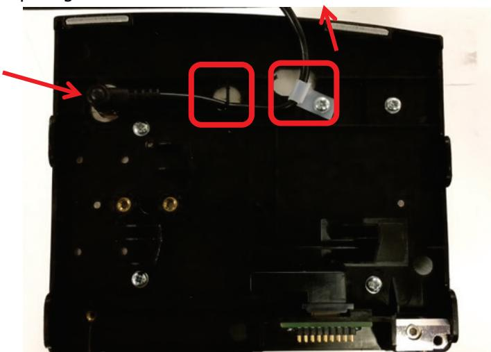
**Figure 3 The power cable connected bottom of the module**
