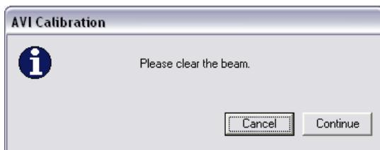
2. Holster the probe, making sure that the Spectralon reference material is in place, and then click **Continue**.
