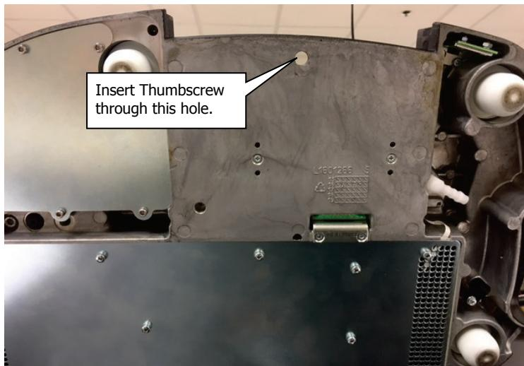
**Figure 4 Thumbscrew location under the Spectrum Two N**
