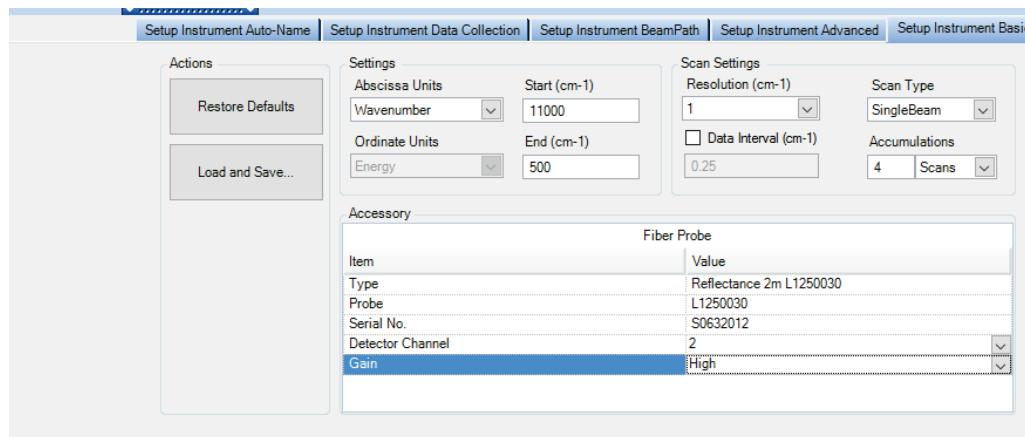
**Figure 11** Setup Instrument Basic tab with Remote Sampling Module Controls
