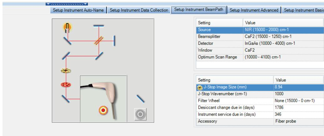
**Figure 12** Setup Instrument BeamPath tab with Remote Sampling Module icon
