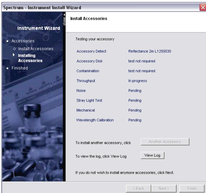
Before beginning the Throughput test, you are prompted to holster the probe.
