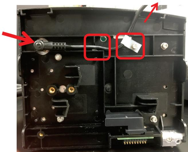
**Figure 4 The power cable connected to HTM**
