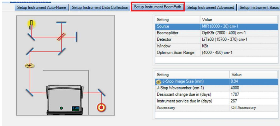
Figure 7 Setup Instrument BeamPath tab with HTM
