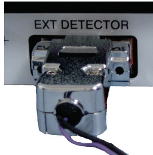
Figure 7 Alignment tool connected to EXT DETECTOR port
