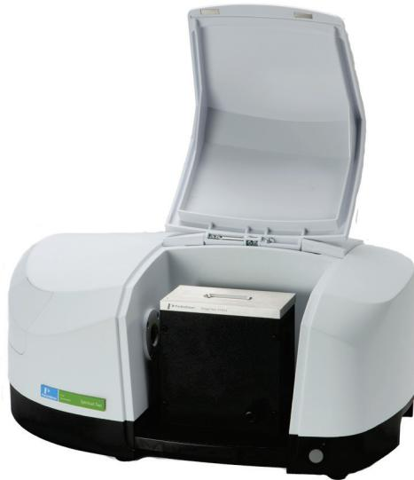
**Figure 1 The Horizontal Attenuated Total Reflectance (HATR) Accessory**
