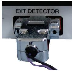
**Figure 8 Alignment tool connected to EXT DETECTOR port**
