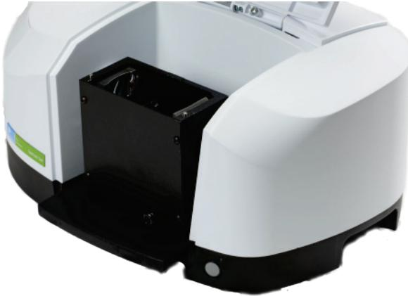
**Figure 4 Installing the HATR accessory**
