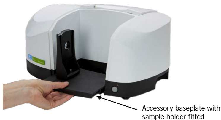
Figure 4 Removing the sampling accessory
