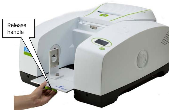
**Figure 2 Removing the Sampling Accessory**
