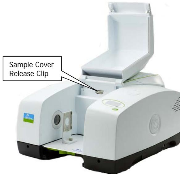
**Figure 1 Removing the Sample Compartment Cover**
