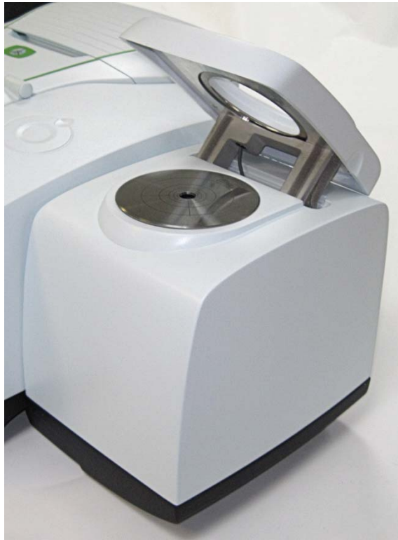
Figure 21 Locating feet of sample spinner in the interface slot
