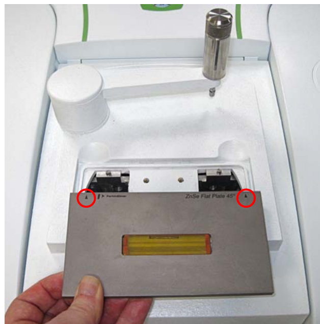
Figure 6 HATR accessory top plate with arrows circled
