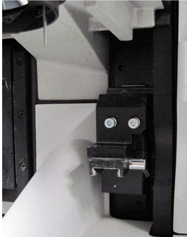
Figure 22 Location of the dovetail connector behind the stage
