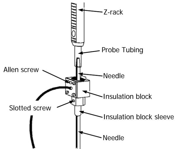
**Figure 22 Connecting the needle tubing to needle**
