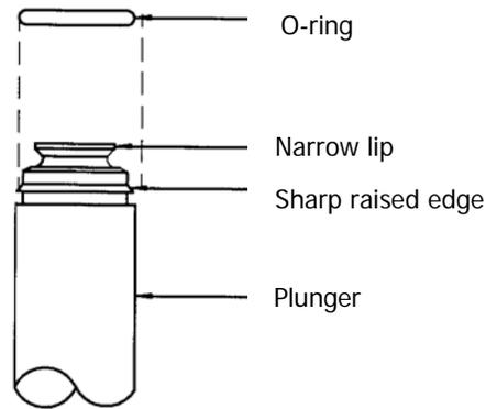
**Figure 30 Plunger and O-ring configuration**
