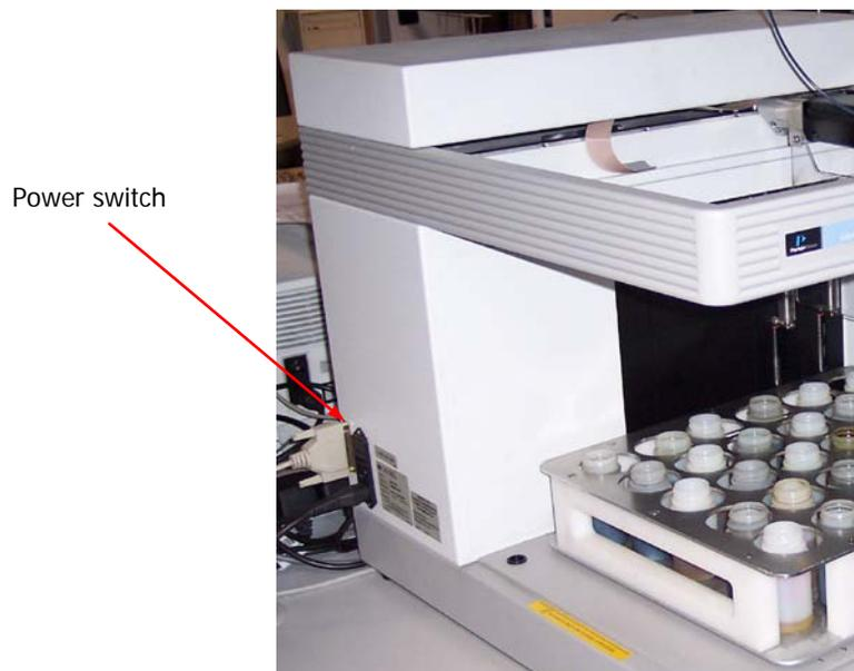
**Figure 2 Location of the Autosampler power switch**
