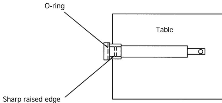
**Figure 31 Seal installation**
