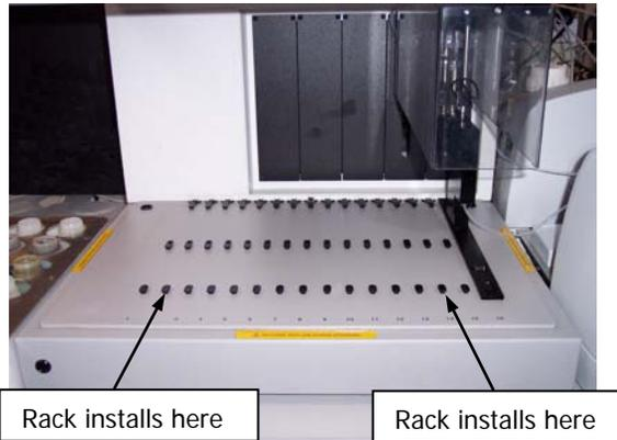
**Figure 18** Installing the sample rack
