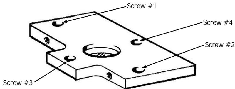
**Figure 35** Flowcell securing sequence
