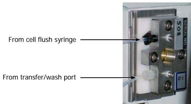
**Figure 20 Connecting tubing to the 2-port flowcell**
