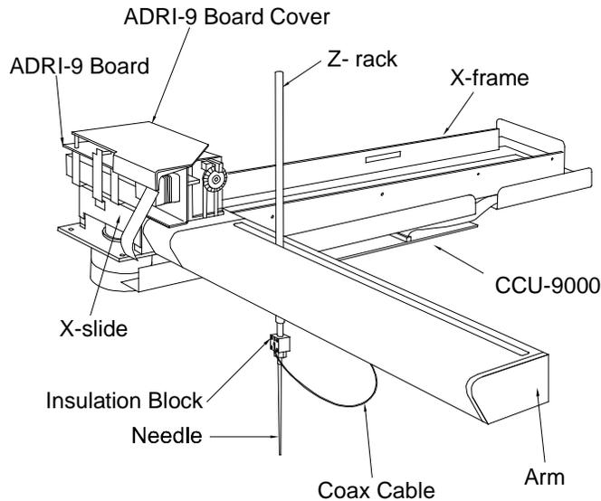
Figure 4 X – Y – Z arm mechanism
