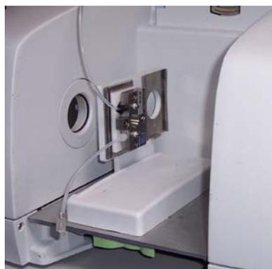
**Figure 24 Sample shuttle accessory and flowcell fitted**
