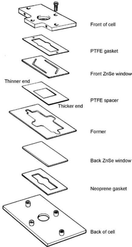
**Figure 34 Dismantling or assembling the flowcell**
