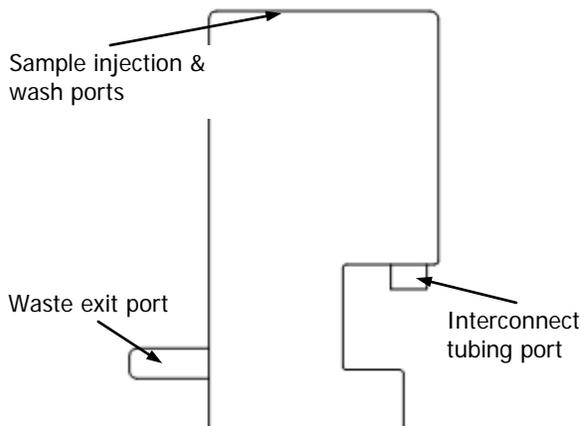
**Figure 6 Sample injection and wash ports (side view)**
