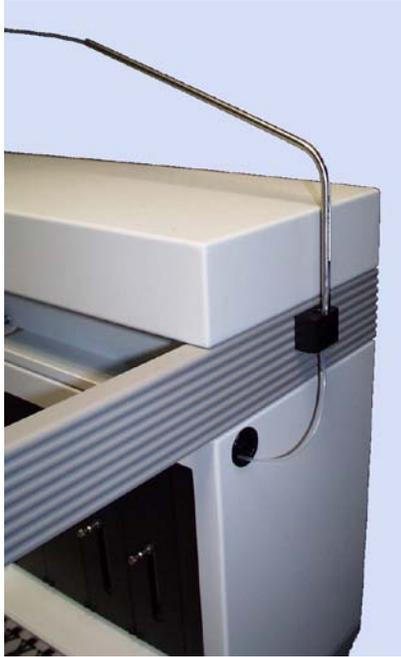
**Figure 17 Fluid line support arm**
