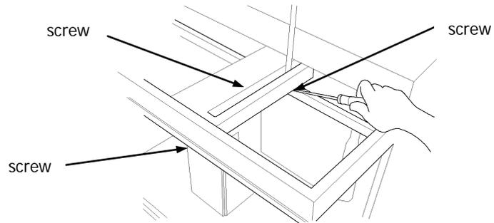
**Figure 26 Installing the arm shield**
