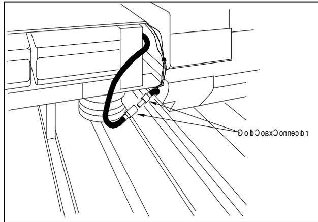
**Figure 33 Disconnecting the insulation block cable**
