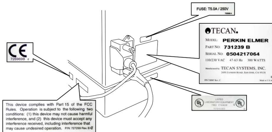
Figure 13 Autosampler labels (rear and left side)
