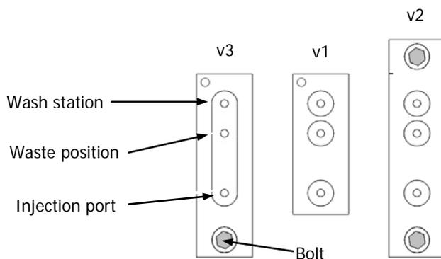
**Figure 7 Sample injection and wash ports (top view)**
