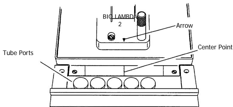
**Figure 10** Installing the single cell holder
