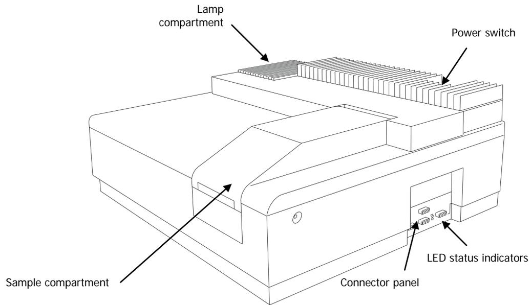
**Figure 5 Lambda 25, 35, 45 spectrometer features**
