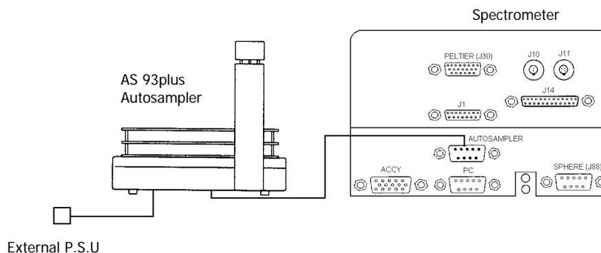
**Figure 16 Connecting to an Autosampler**
