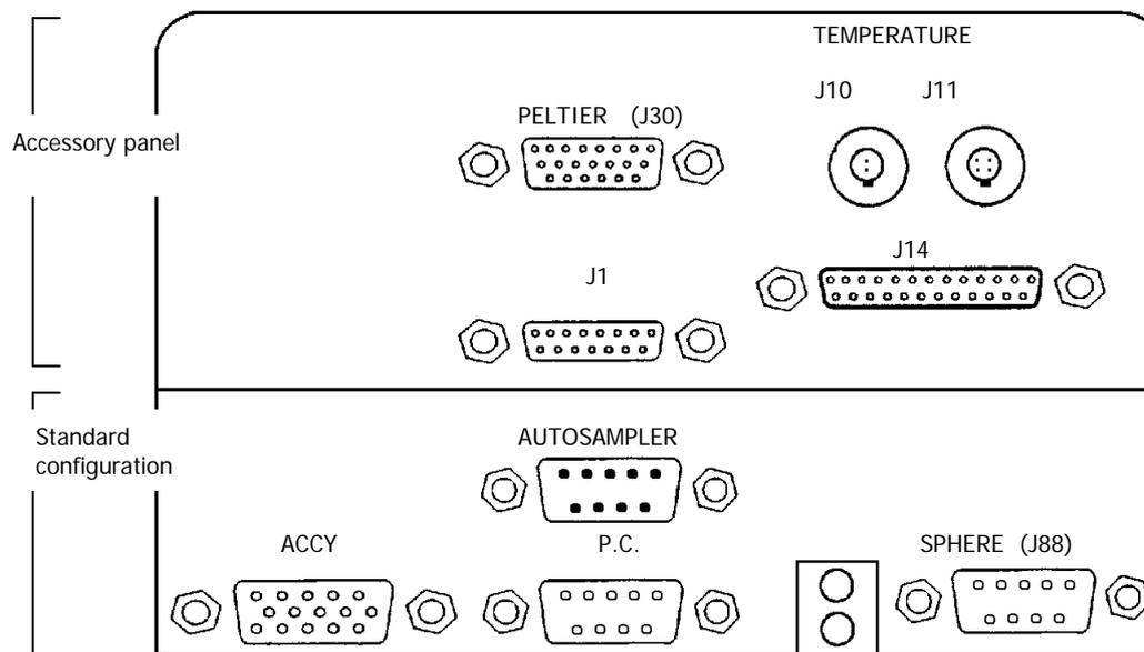
Figure 13 Accessory connector panel
