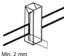
**Figure 11 Correct alignment of the radiation beam in the cell sample area**
