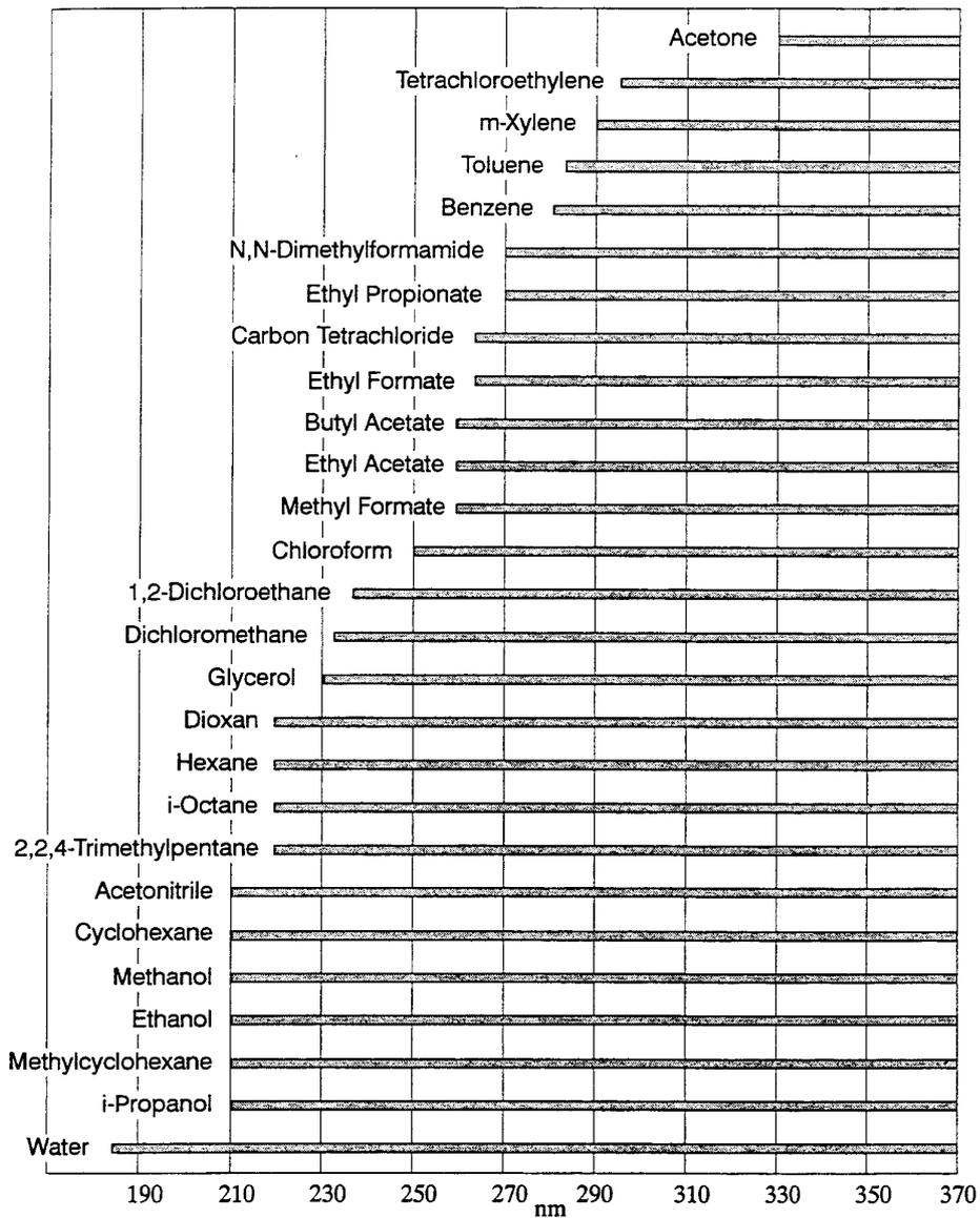
Figure 29 Lower wavelength limits of solvents
