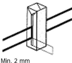
**Figure 12 Correct alignment of the radiation beam in the cell sample area**
