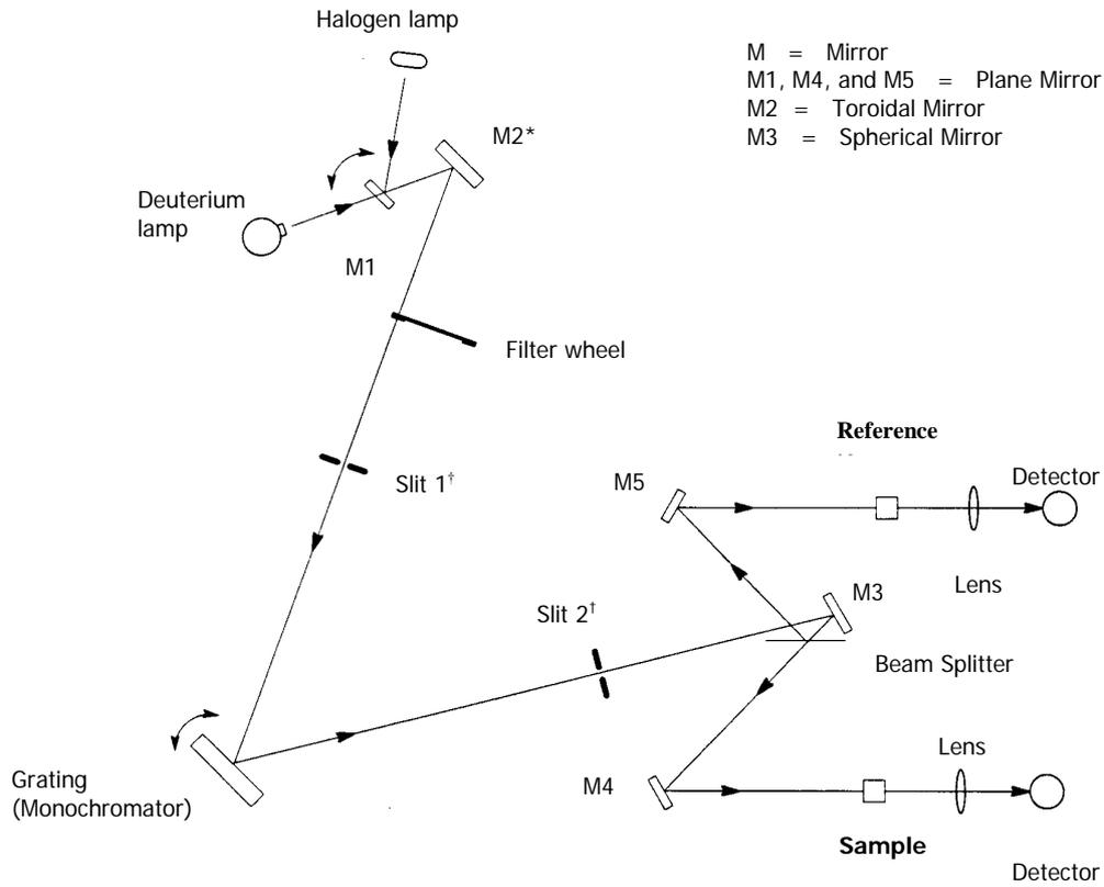
**Figure 6 Optical path for Lambda 25, 35, 45**
