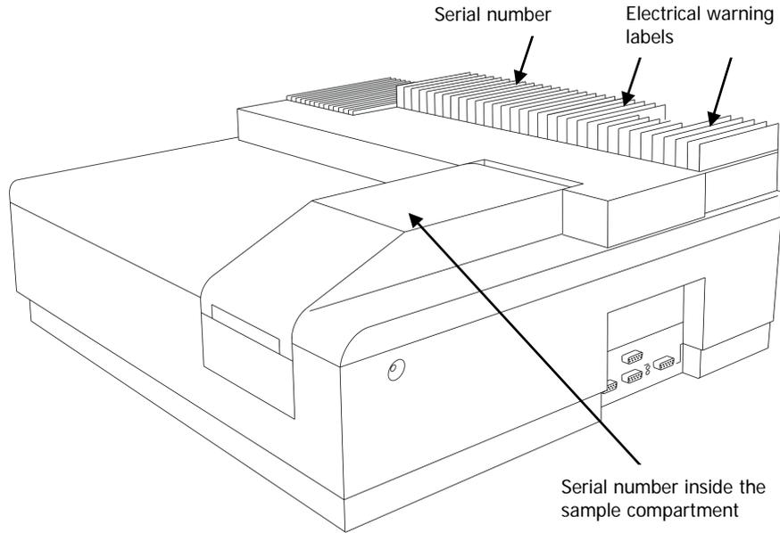
**Figure 1 Labels on the spectrometer housing**
