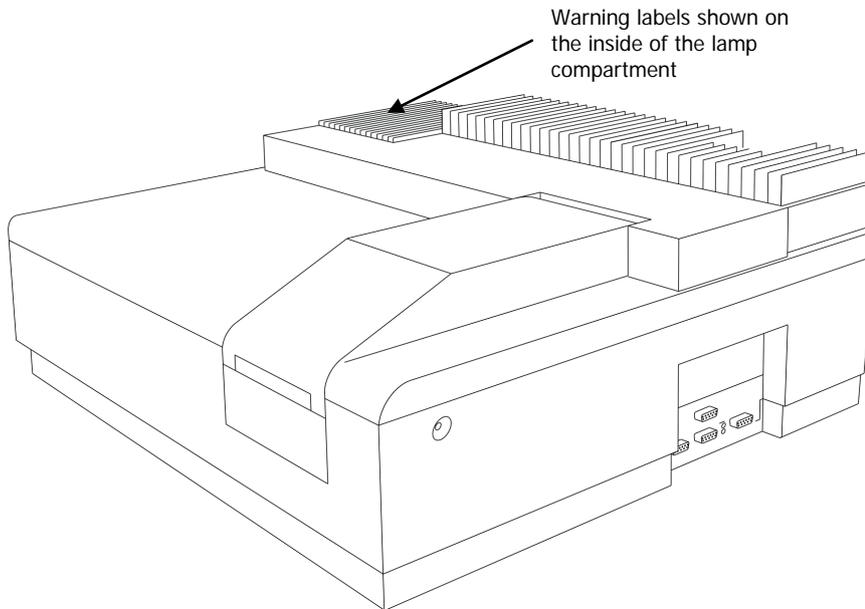
Figure 3 Lambda 25, 35, 45 Spectrometers warning labels (inside lamp compartment)
