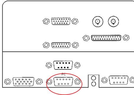
**Figure 8 Connecting the PC to the spectrometer**
