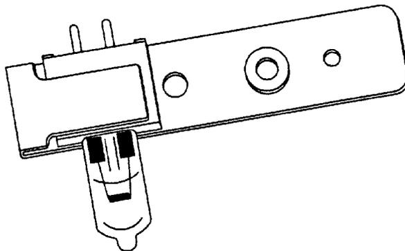
Figure 19 Pre-aligned halogen lamp (B0114620)
