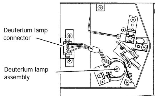
**Figure 24 Deuterium lamp connector**
