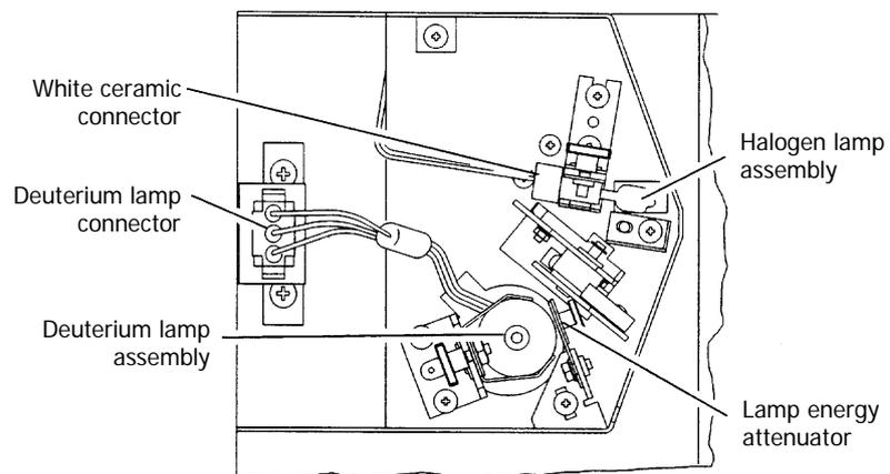
**Figure 18 Inside the lamp compartment (baffle removed)**
