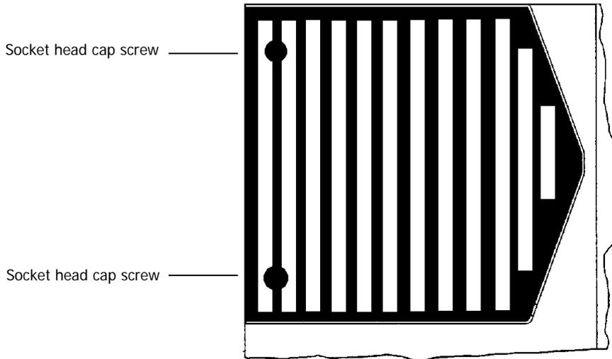
**Figure 25 Lamp baffle**
