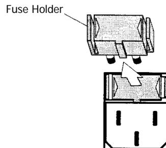
**Figure 28 Removing the fuse holder**
