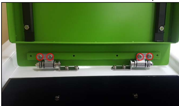
Figure 10 Remove the sample compartment lid
