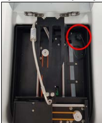
Figure 16 Accessory fixing bolt of Microplate Reader
