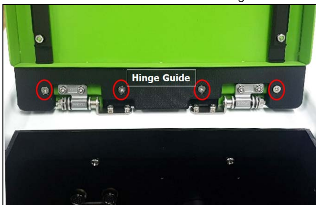
Figure 9 Remove the Hinge Guide
