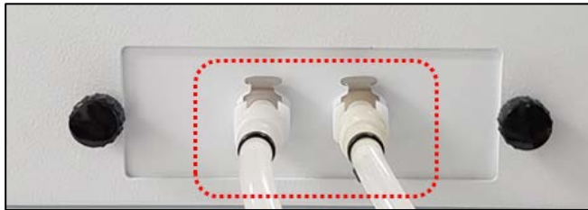
Figure 11 Connecting the male connector to the quick coupling
