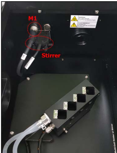
Figure 9 Insert the M1 and Stirrer cables
