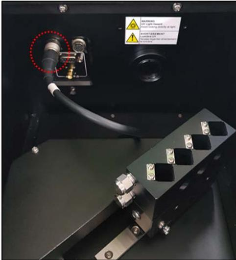
**Figure 6 Connect the M1 cable**
