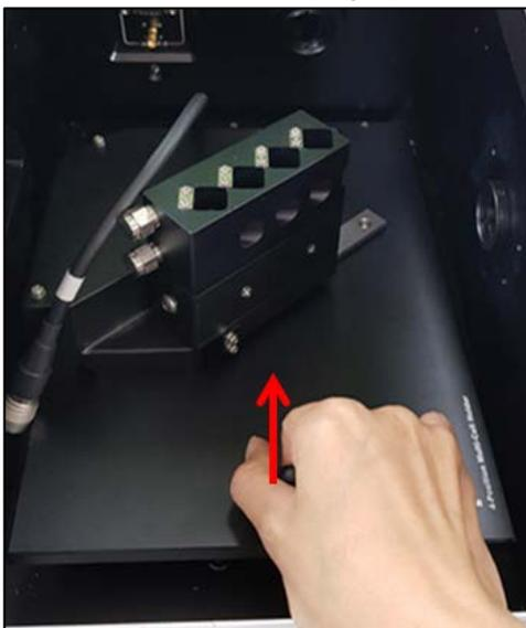
**Figure 5 Installing the accessory**
