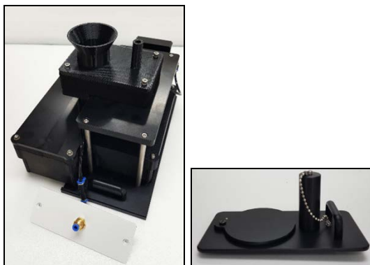
Figure 1 Low Temperature Cell Holder (P/N:N4201045)
