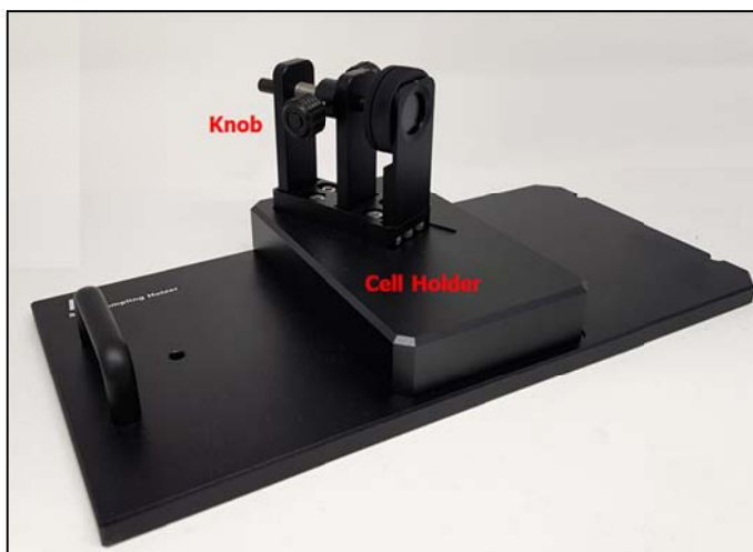
Figure 2 Solid Sample Holder Configuration
