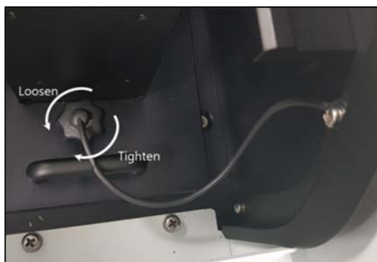
Figure 3 Loosening the Accessory Fixing Bolt
