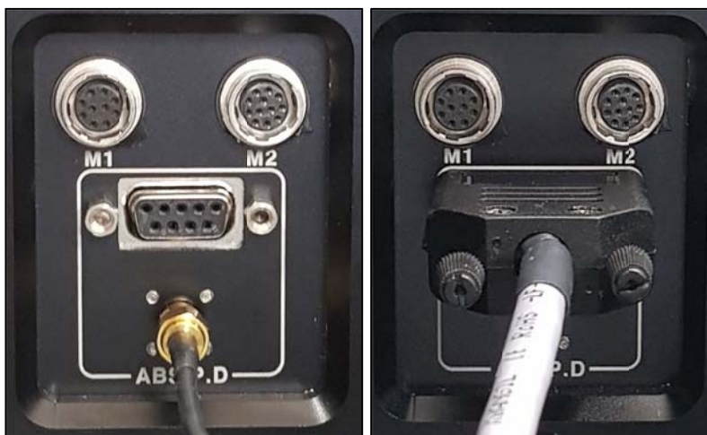
Figure 7 Connecting the SMA Connector and Absorbance Module Power
