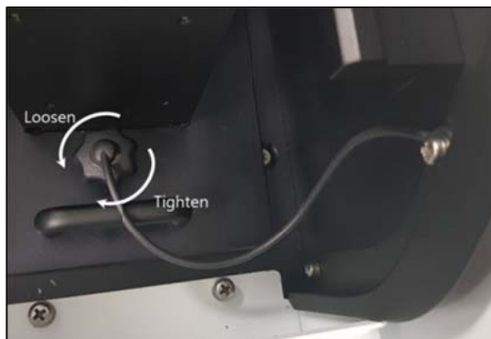
Figure 6 Tightening the Accessory Fixing Bolt
