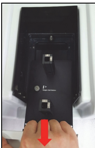
Figure 15. Pulling out the cell holder and base plate
