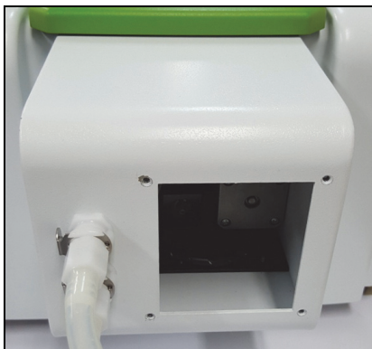
Figure 21. Removing the Plate for Calibration
