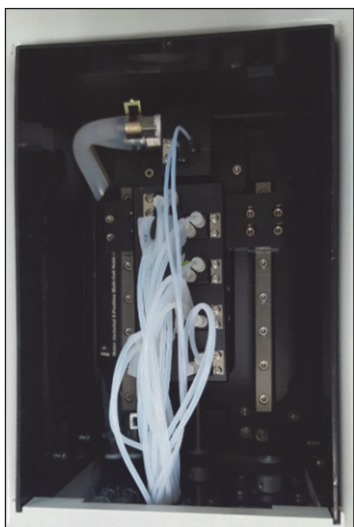
Figure 25. Inserting flow cells
