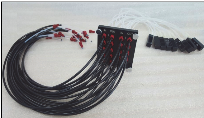
Figure 22. Manifold with all the tubing connected
