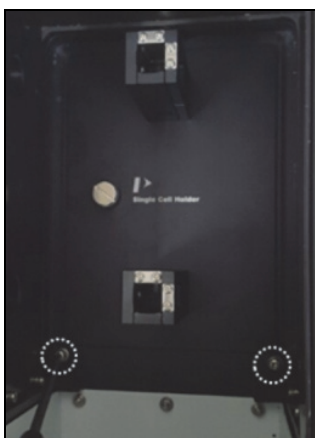
Figure 14. Location of the round head screws with washer
