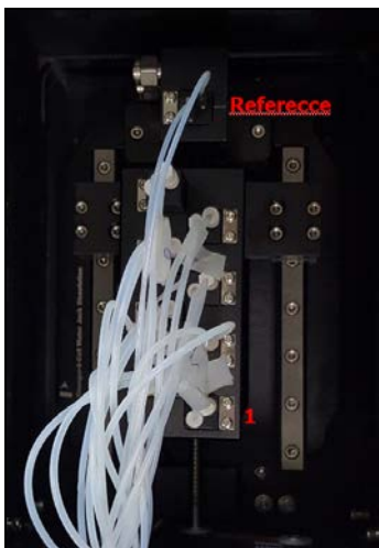
Figure 28. Inserting No.1 and reference cells into the cell holder
