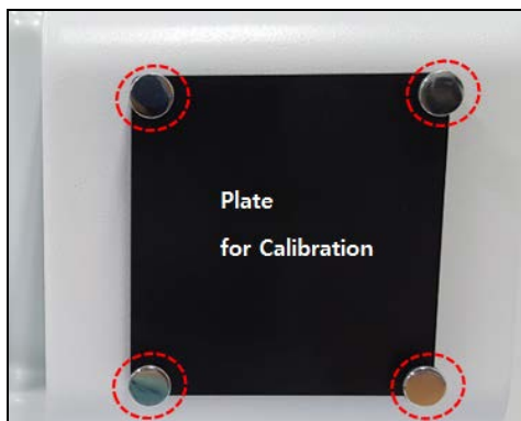
Figure 18. Tighten the 4 bolts
