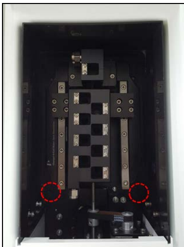
Figure 17. Tighten the Changer 8-Cell for Dissolution
