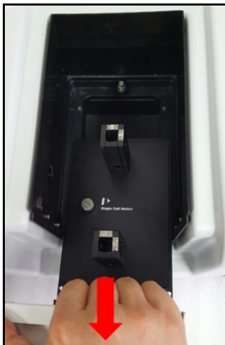
Figure 14. Pulling out the cell holder and base plate
