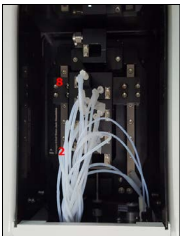
Figure 25. Inserting cells from 2 to 8
