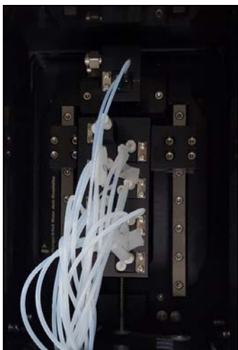
Figure 23. Inserting flow cells
