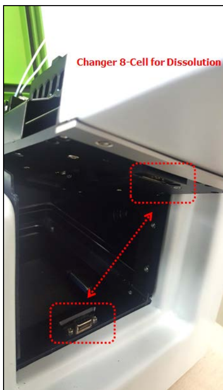
Figure 16. Connecting the communication ports
