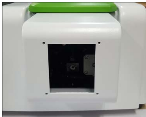
Figure 19. Removing the Plate for Calibration
