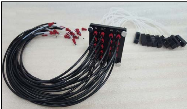
Figure 20. Manifold with all the tubing connected
