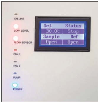
Figure 22 LEDs of LOW LEVEL and FLOW SENSOR
