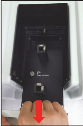
Figure 24 Pulling out the cell holder and base plate
