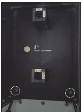
Figure 23 Location of Phillips round head screws with washer
