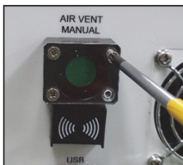
Figure 17 Removing Phillips screws
