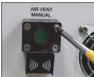
Figure 10 Removing Phillips screws
