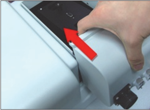
Figure 25 Inserting the Single cell peltier holder
