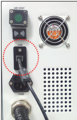
Figure 32 Connecting the Peltier Temperature Controller 201 with the PC
