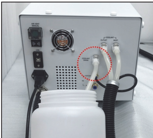
Figure 21 Connect the waste hose
