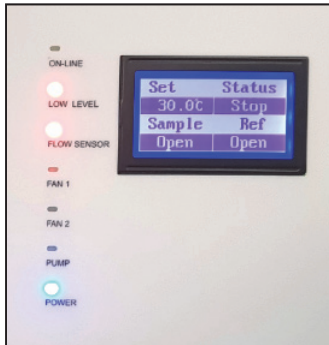
Figure 22 LEDs of LOW LEVEL and FLOW SENSOR
