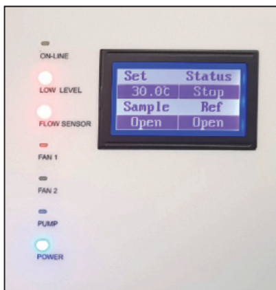
Figure 13 LEDs of LOW LEVEL and FLOW SENSOR
