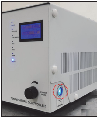
Figure 20 Turn on the AC power switch
