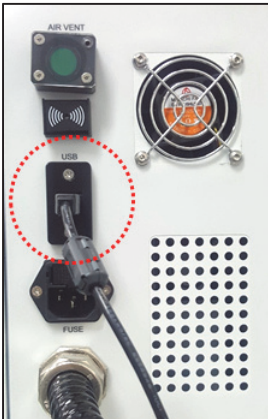
Figure 34 Connecting the Peltier Temperature Controller 201 with the PC
