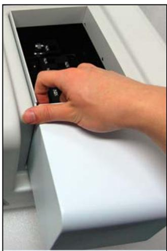
**Figure 8 Inserting the 5-Pos Variable Pathlength Cell Holder in the sample compartment**
