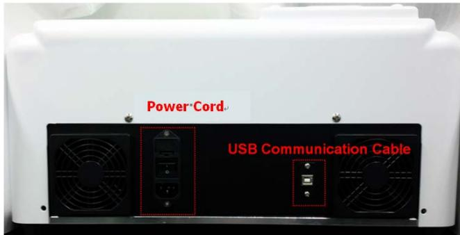
**Figure 5 Connecting the power cord and USB communication cable**
