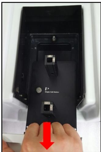
**Figure 7 Pulling out the cell holder and base plate**
