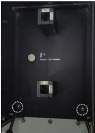
**Figure 6 Location of the two Phillips round head screws with washer**
