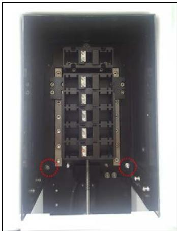
**Figure 10 Tighten the 5-Pos Variable Pathlength Cell Holder in the sample compartment**
