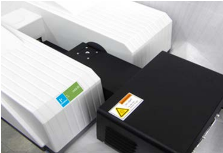
Figure 4 Installing the DRA-100
