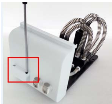
Figure 17 Detaching the Stirrer cable fixing block
