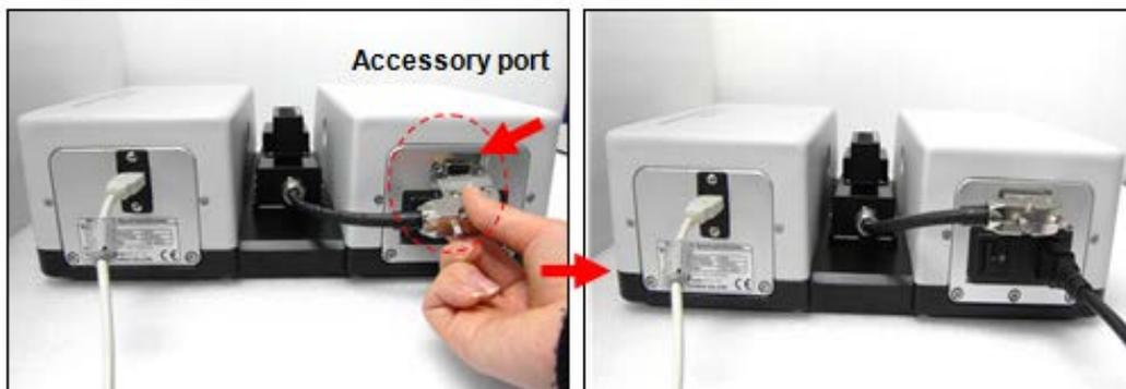
Figure 6 Connecting the accessory communication cable to the accessory port
