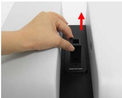
**Figure 4 Removing the existing cell holder**
