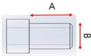
**NOTE:** The recommended tube size and material are 4 mm-ID and 8 mm-OD silicon tube which has thermal resistance at higher than 100°C
