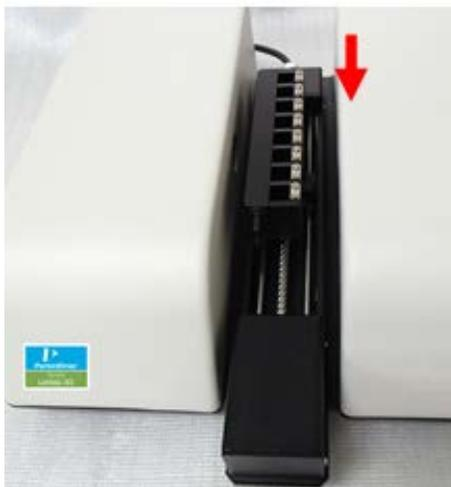
**Figure 5 Water Jacketed 8-Position Multi-Cell Holder (or 8-Position Multi-Cell Holder)**
