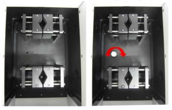
Figure 7 Inserting the test tube holder
