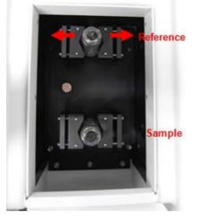
Figure 8 Inserting the test tube holder
