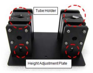
Figure 2 Lambda 365 Test Tube Holder Configuration
