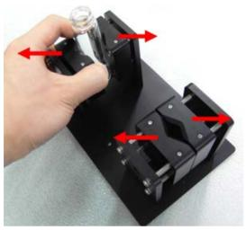
Figure 9 Inserting the test tube When the tube height is more than 105 mm
