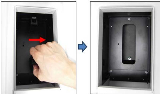
**Figure 7 Pulling out the cell holder**
