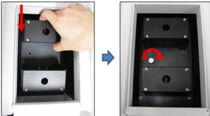
**Figure 8 Inserting the Fixed Angle Reflectance Holder**
