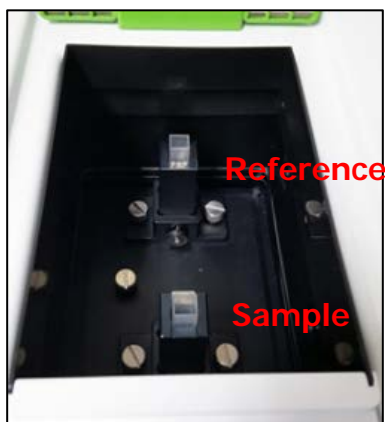
Figure 7 Inserting the micro cells into the cell holder
