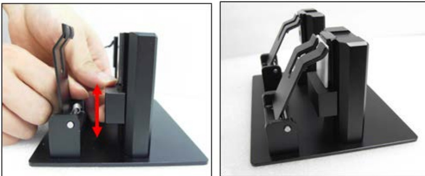
Figure 9 Controlling the height
