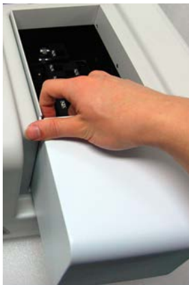
Figure 7. Inserting the 8-Position Multi-Cell Holder in the sample compartment
