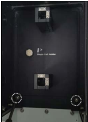
Figure 5 Location of the two Phillips round head screws with washer
