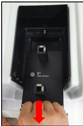
Figure 6 Pulling out the cell holder and base plate
