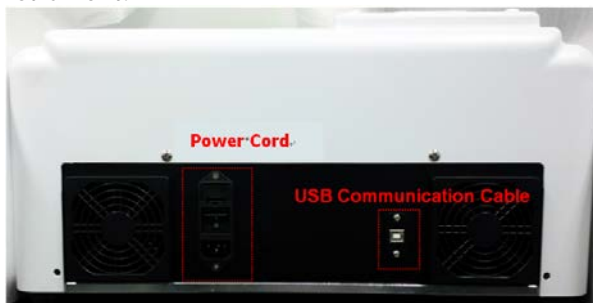
Figure 4 Connecting the power cord and USB communication cable
