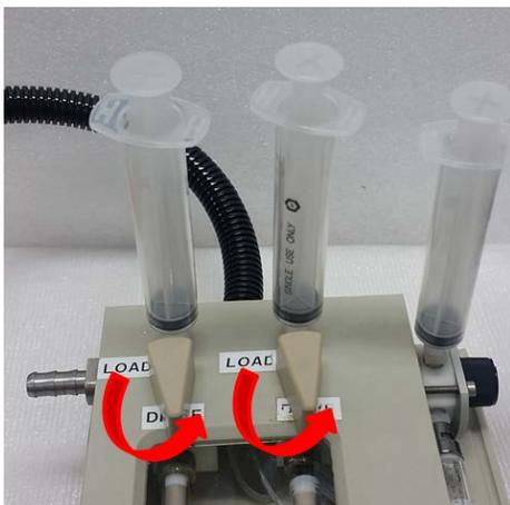
**Figure 13 Placing valve at the DRIVE**
