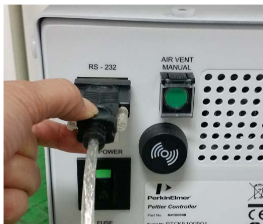
Figure 12 Connecting the Peltier Controller
