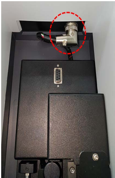
Figure 8 Connecting the Peltier 8-pin cable of the Peltier control Multi-Cell to the port of the main board
