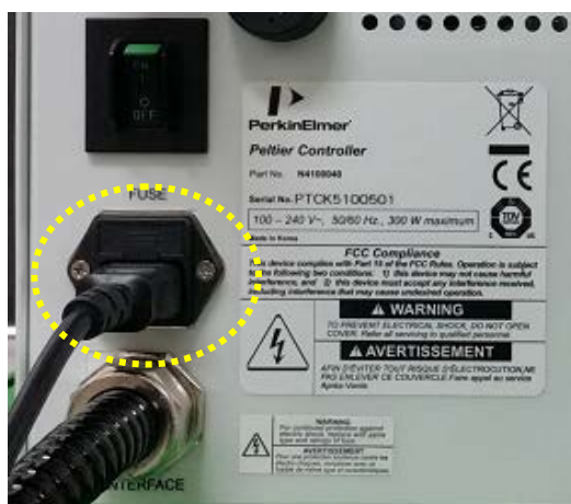
Figure 13 Connecting the power cord
