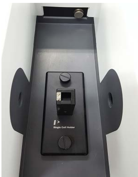
Figure 6 Taking apart the existing cell holder
