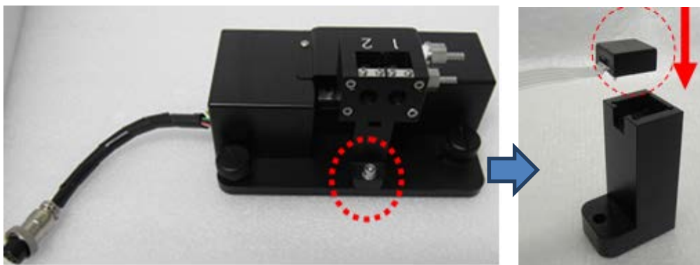
Figure 7 Placing the Magnetic Stirrer Head on the Stirrer Mount
