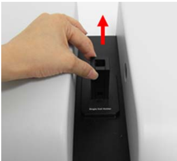
Figure 4 Removing the existing cell holder
