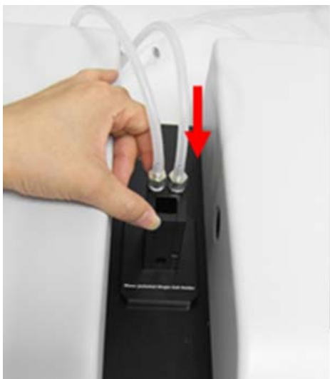
Figure 6 Installing the water jacketed single cell holder
