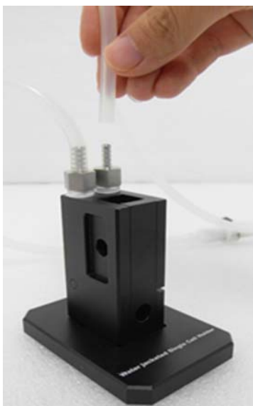
Figure 5 Connecting the tube to the hose fitting
