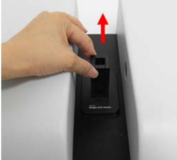
Figure 3 Removing the existing cell holder
