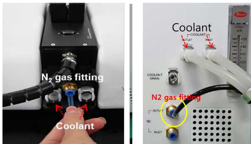
Figure 9 Connecting the coolant inlet/outlet and N_2 gas tube
