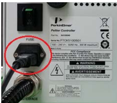
Figure 12 Connecting the power cord to the Peltier controller
