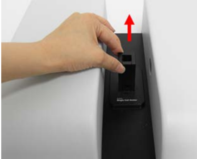
Figure 6 Removing the existing cell holder
