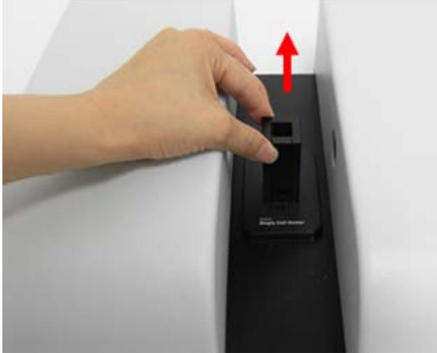
**Figure 3 Removing the existing cell holder**
