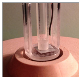
Figure 2. Expansion probe on can liner sample
