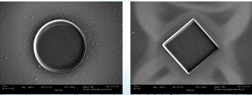
Using a proprietary component to enable maximum beam homogenization the Analyte Excite system is able to generate beautiful flat bottomed craters with sharp edges and with no visible melting. The 50 µm circle (left) is the result of 10 ablation shots, and the 80 µm square (right) is from a 25 shot ablation.
